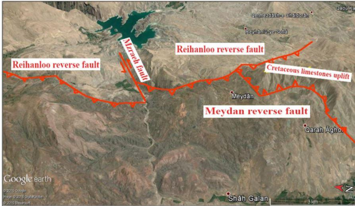
Fig. 10. Reihanloo reverse fault, which has caused limestone and marls thrusting of Qom Formation on ophiolite rocks.
